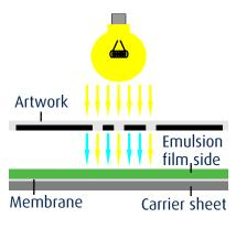
**NOTE:** Overexposure can cause image not to washout. Underexposure can cause entire mask to washout prematurely.
