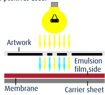
**NOTE:** Overexposure can cause image not to washout. Underexposure can cause entire mask to washout prematurely.
